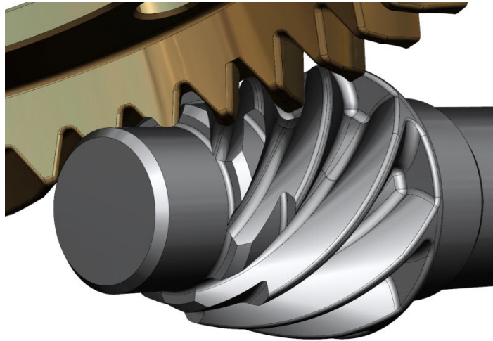
Fig. 3. Increase of the bending strength of the pinion with design improvement on the tooth heel is possible only if CNC tooth cutting is used
