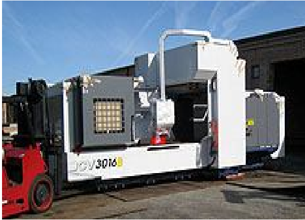
Fig. 1. 3-axis universal CNC milling machine with 1800 x 2500 mm table for $500,000.00US
