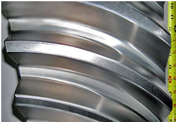
Fig. 2. Case hardened Metso MP 1000 gear finished on 3-axis universal CNC milling machine using ten new 12mm ball-end milling cutters ($30.00 each). Dimensions on the picture are in inches
